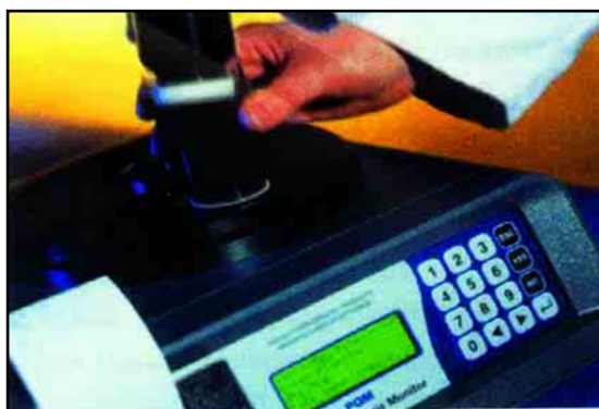
Kittiwake's AnalexPQ magnetometer measures the mass of ferrous-wear debris in oil samples
